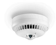
Thermal detector with fixed and rate of rise temperature settings for Loop 3000 with two thermal sensors for earliest fire detection and indication in all environments with difficult ambient conditions and with bidirectional isolator, according to EN 54-5 and EN 54-17
